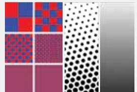
Dithering, or halftone printing, produces a continuous tone effect at a sufficient viewing distance, forming gradients
