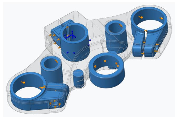
*Easily set up optimization by defining the design space, physics, loads and constraint goals, manufacturing process and materials.*
